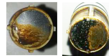
Fig.: Coupons partially shielded by an inhibiting film
