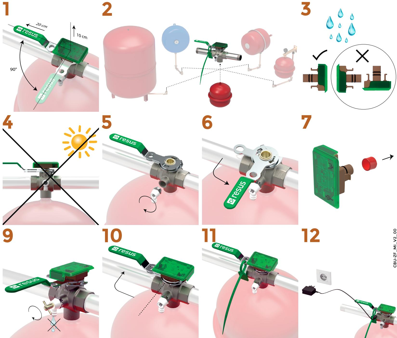
**NORMAAL GEBRUIK** in retour naar warmtegenerator / **NORMAL USE** in the return line to the heat generator
