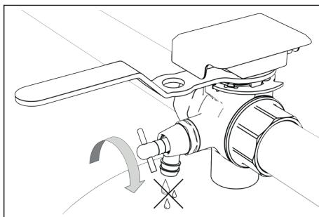
7. Turn the lever 90° clockwise into its normal operating position (= full bore).
