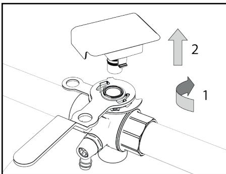
6. A new corrosion monitor can now be mounted as described from step 3 for installation in *Chapter 6, Installation*.
