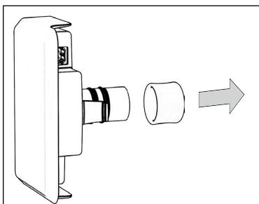
5. The corrosion monitor may then be placed in the fixture by means of bayonet mounting. Be careful not to damage the probe tip when inserting.
