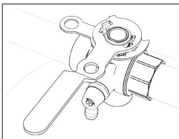
4. Remove the protective cap from the probe.
