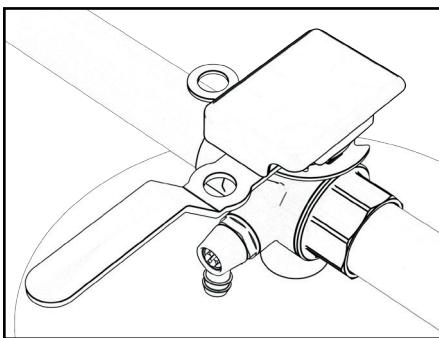
4. Connect a hose to the hose connector, and open the drain valve to completely empty the expansion vessel.
