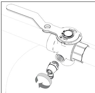
3. Turn the lever of the lockshield valve device perpendicular relative to the pipeline.
